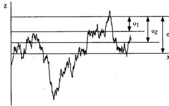
Fig. 3 Fractal surface profile intersected by two planes below the r.m.s. height \sigma
